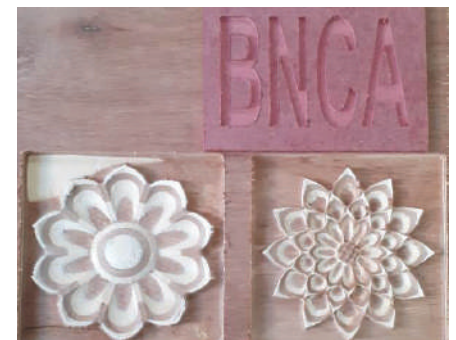
Samples of milling of variable depths
