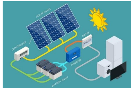
Figure 1: solar panel working diagram ( https://blog.livguard.com/2023/04/maximize-savings-and-sustainability-with-home-solar-power-systems-in-india/ )
