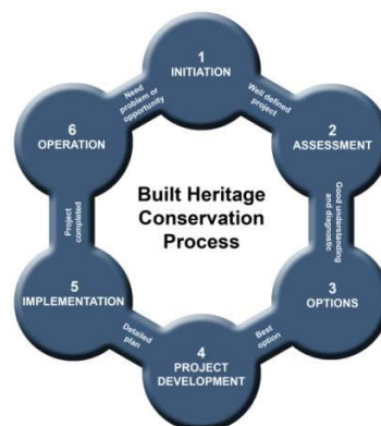
Figure 3: Six phases of the built heritage conservation process and their outputs (Source: http://ip51.icomos.org/fleblanc/publications/pub_2007_conservation_process )
