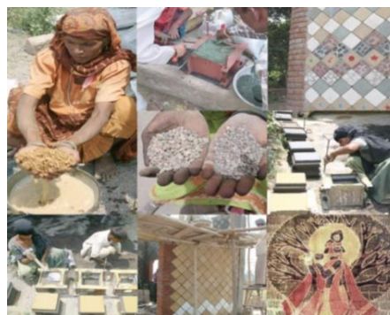
Figure 8. Steps for making Paper Mache blocks hollow core interlocking blocks
