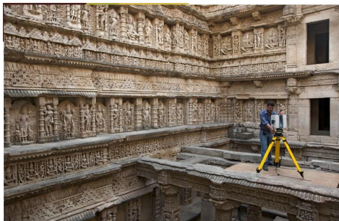
Figure 2: Rani ki Vav – documentation on site by LIDAR
